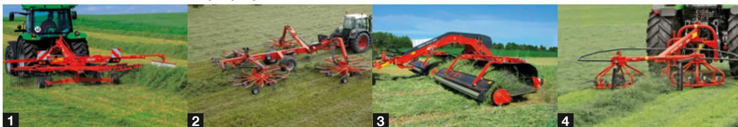
1. Suspended monorotors - 2. Semisuspended with 4 rotors - 3. Harrows of belts - 4. Combined harrow/henifier machines
